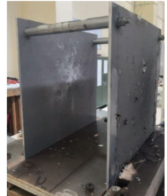
Hyper-velocity Impact tests on MMOD protection shield
